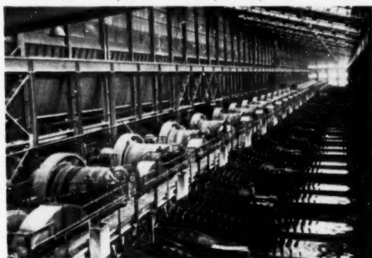
27—10' x 10' Marcy Grate Discharge Mills grinding in excess of 50,000 tons per day in large western copper mill.
